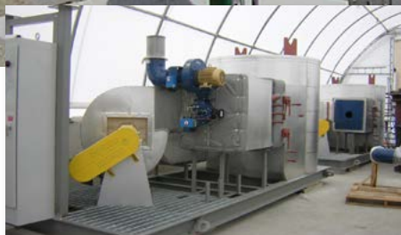
Model RBO Recirculation Fan for Melting Plastic
