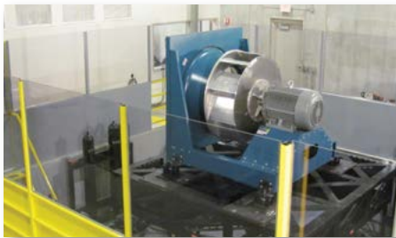
Seismic testing for fans up to 10,000 pounds
