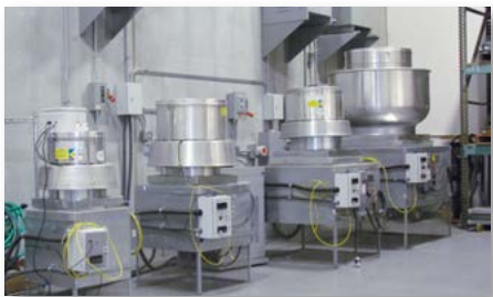
UL 705 safety testing for fans
