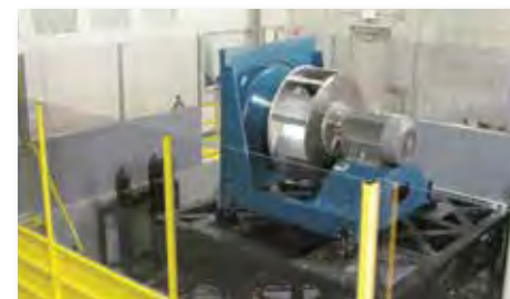
Seismic testing for fans up to 10,000 pounds
